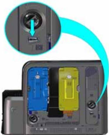
3. Reach into the flipper module and rotate it until you can access the card.
