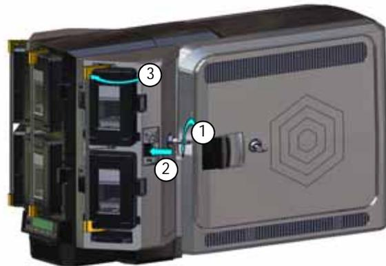
4. Press the cartridge release button at the top of the cartridge and open the cartridge door.
