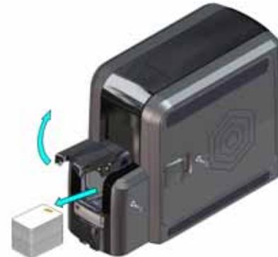
6. Insert the cleaning card into the input hopper.
